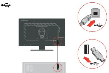
**Note:** The USB port will stay in function as long as the monitor is connected to power, regardless of whether the monitor is switched on or off.
